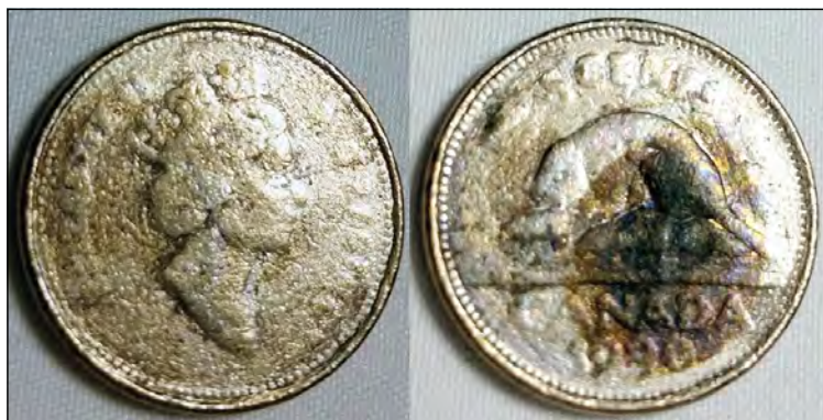
Figure 6. How did grease manage to cover the high and incused parts all over the dies on both sides?
