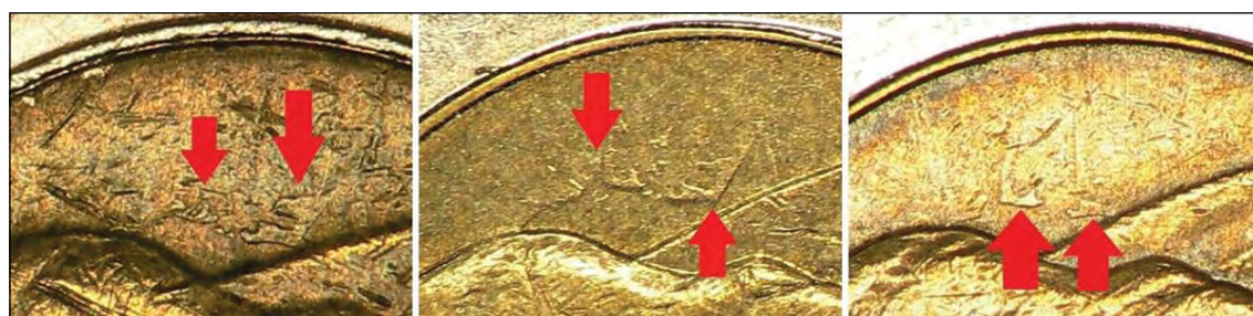
Illustration 9. The illustrations of three different 1996 toonies proves clashed dies were involved in their production.
