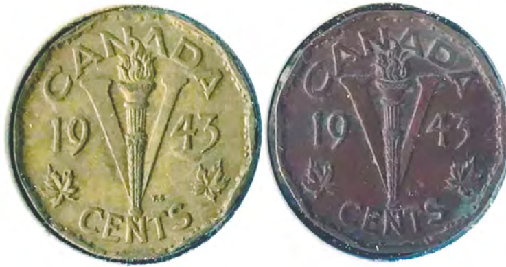
Illustration 2. The transformation in the appearance from normal (left) to dark is most likely due to oxidization.
