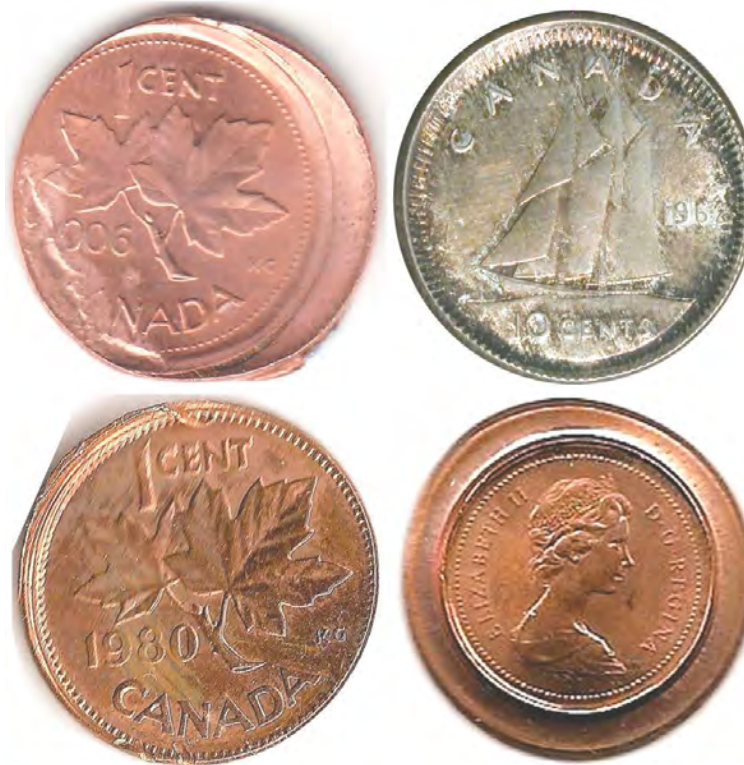
Illustration 2. The off-centre, broad-strike, high rim, die cap and railroad wheel rim, although normal, would be errors with reverse die set-ups if they had more recent dates.
