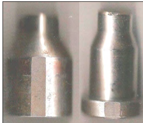
Illustration 4. The bottom (reverse design) dies used at the Denver Mint contain a flat notch.
