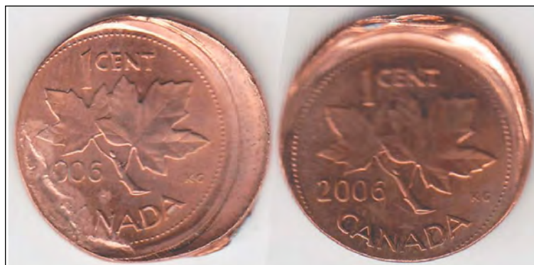
Illustration 1. The off-centre can be in any direction regardless which way the dies are facing.
