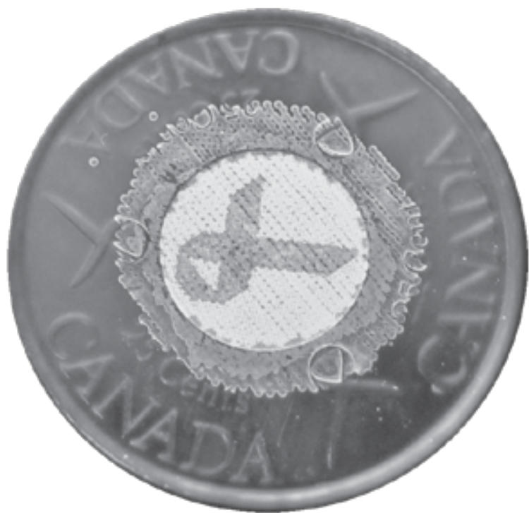
Figure 5. A 2006 Pink Ribbon 25-cent coin under UV light shows coating of a large area.
