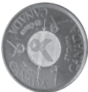
Figure 6. The thick line is the result of two halves of white 'spray' overlapping.
