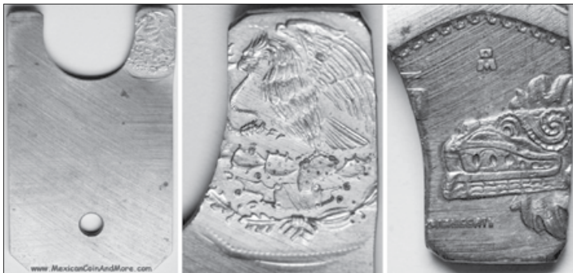
Figure 3. This finger from an old-style mechanical finger feed press struck by a 5-peso coin can be had for $5,375. Shown is one side of the finger and blow-ups of both sides of the portion struck by the dies.
